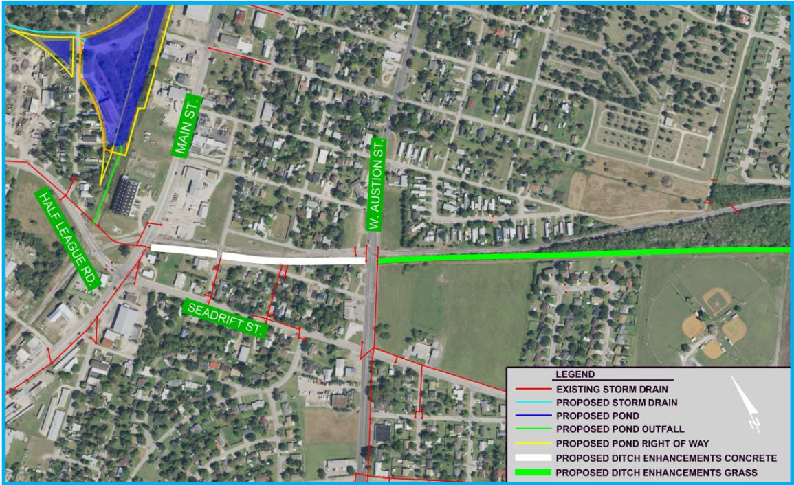
Figure 3.3 Proposed grass/overgrown ditch enhancements.
